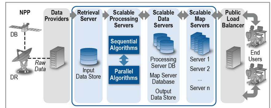
**Figure 2: NPP Product Generation Cloud Computing Architecture**
